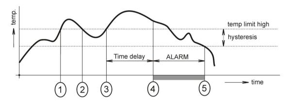
An alarm report is always sent right after an alarm appears. The device memorizes sent alarm reports of current alarms while the power is connected. In case of power disconnection or a reset of the device (e.g. by modification of configuration) a new alarm evaluation is performed and new alarm reports are sent again, if any.
